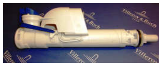
Bottom feed filling valve NOTE-New style cistern 1/2" required Old style 10yrs + 3/8" required which is copper
